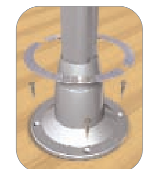
Permanent floor fixing
